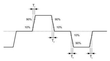
Figure 5-2 - 100Base-TX  $T_{r/f}$  Timing
