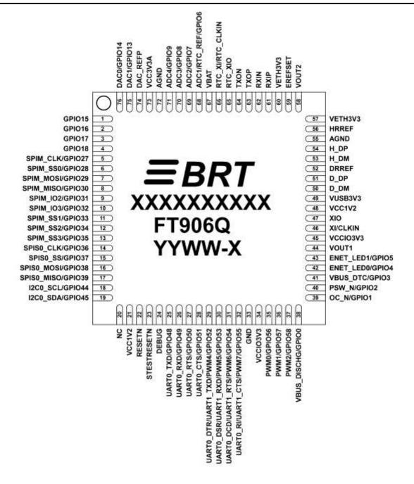
Figure 3-2 - Pin Configuration FT906Q (top-down view)
