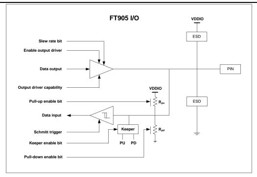
Figure 6-5 - Standard I/O pin configuration
