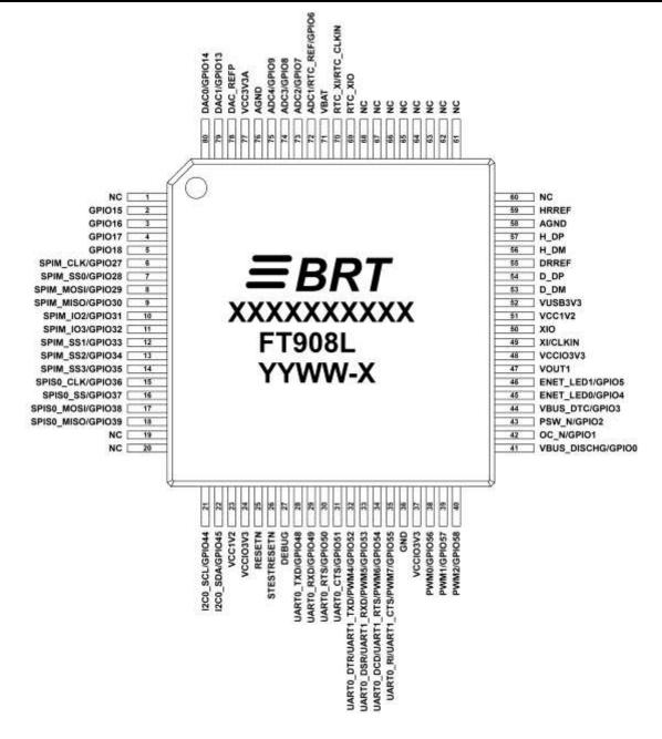
Figure 3-8 - Pin Configuration FT908L (top-down view)
