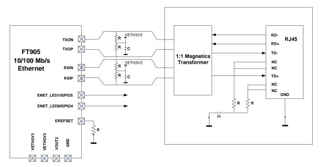
Figure 6-7 - 10/100 Mb/s Ethernet interface
