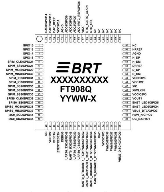
Figure 3-4 - Pin Configuration FT908Q (top-down view)
