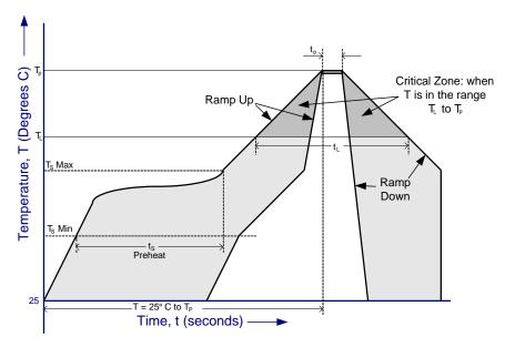
Figure 7-5 - FT905 Solder Reflow Profile
