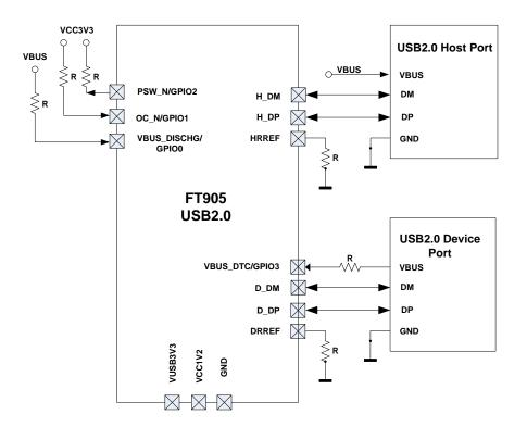
Figure 6-6 - USB 2.0 ports connection
