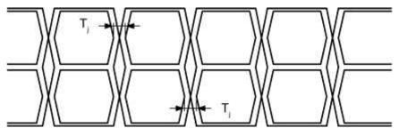
Figure 5-3 - 100Base-TX Jitter Timing
