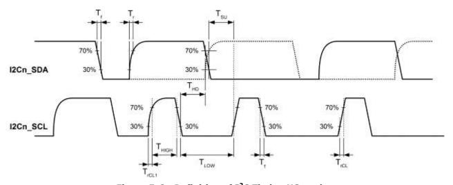
Figure 5-6 - Definition of  ${\bf I}^2{\bf C}$  Timing HS mode
