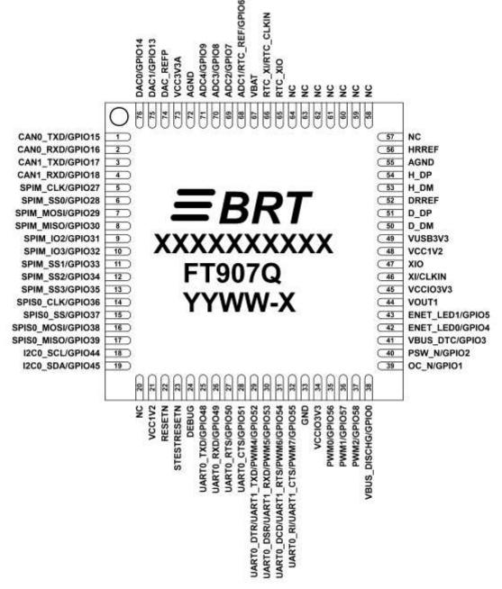
Figure 3-3 - Pin Configuration FT907Q (top-down view)
