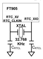
Figure 6-3 - RTC 32.768 KHz oscillator connection
