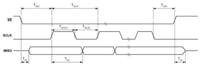
Figure 5-8 - Definition of SPI Slave Timing Mode 0
