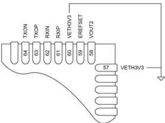
Figure 6-8 - Unused Ethernet Connection (QFN)
