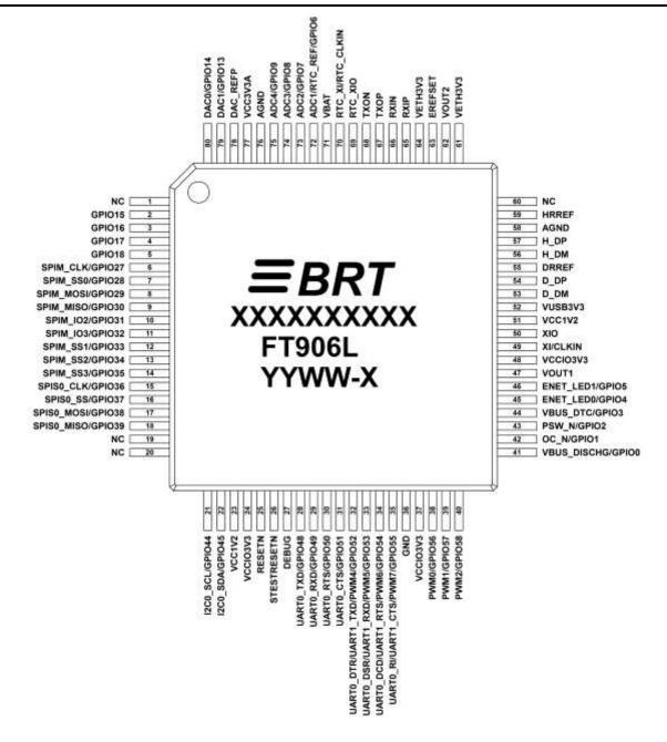
Figure 3-6 - Pin Configuration FT906L (top-down view)
