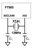
Figure 6-1 - Crystal oscillator connection
