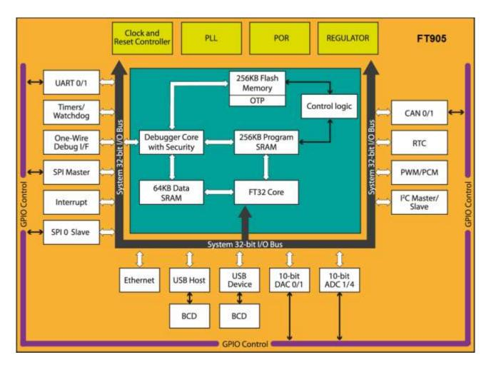
Figure 2-1 - FT905 Block Diagram
