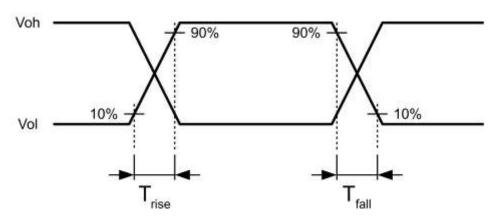
Figure 5-1 - USB Rise and Fall Times for DP/DM
