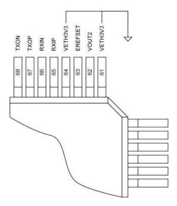
Figure 6-9 - Unused Ethernet Connection (LQFP)
