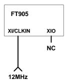
Figure 6-2 - External clock input
