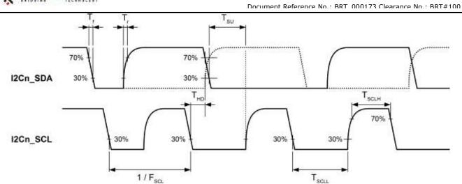
Figure 5-5 - Definition of I<sup>2</sup>C Timing F/S mode
