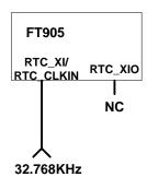
Figure 6-4 - External 32.768 KHz clock input
