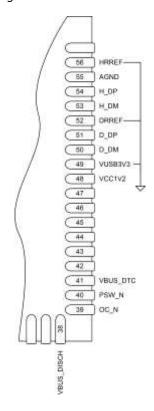
Figure 6-10 - Unused USB Connection (QFN)
