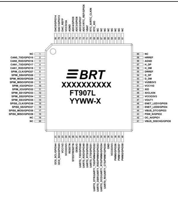
Figure 3-7 - Pin Configuration FT907L (top-down view)
