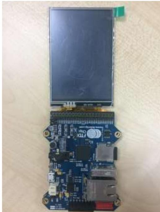
**Figure 9 - Connections between FT900 & FT8xx Modules**
