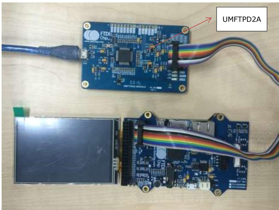
**Figure 7 - Connections between MM900EV2A & UMFTPD2A Modules**
