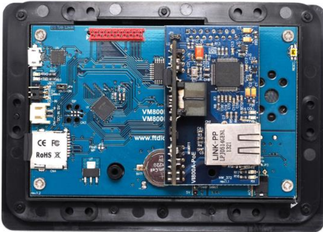
Figure 5-1 – VI800A-PoE module connected to VM800P Plus module
