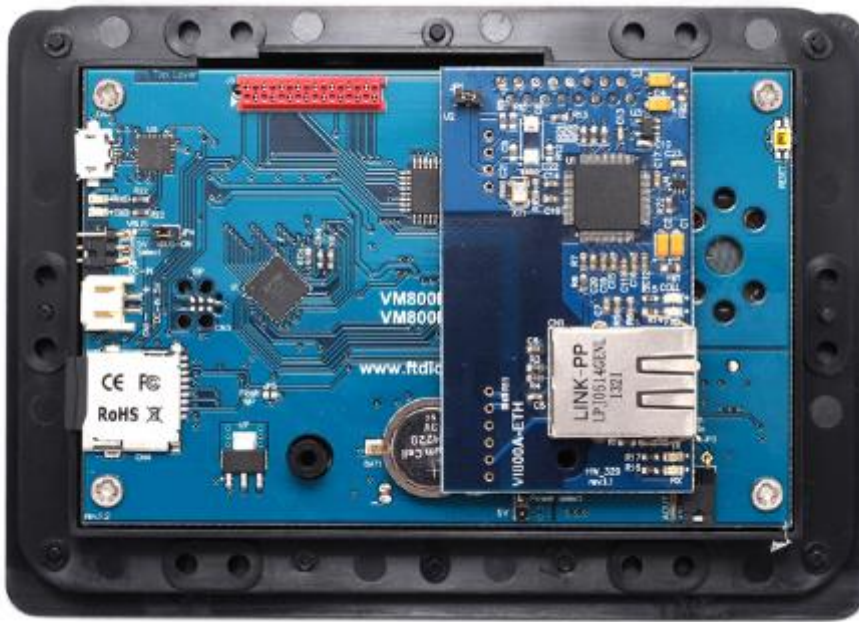
Figure 6-1 – VI800A Ethernet module connected to VM800P Plus module
