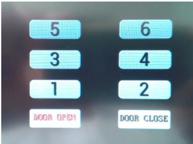
Figure 4.2 The "DOOR OPEN" button is pressed and plays back a "door opening" audio file
