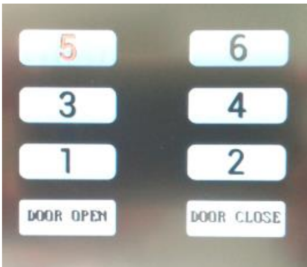
Figure 4.3 The "5" button is pressed and plays back a "5th floor" audio file
