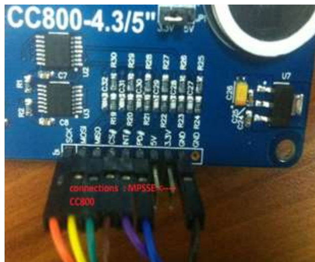
Figure 5 - MPSSE Cable Connection
