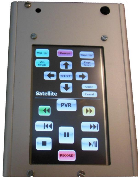
Image 1: This is a touch-screen multi-function IR remote control I built a while back, using 4D Systems uLCD-43PT intelligent TFT touchscreen module. I am now designing a similar device using the much less expensive EVE display modules.
