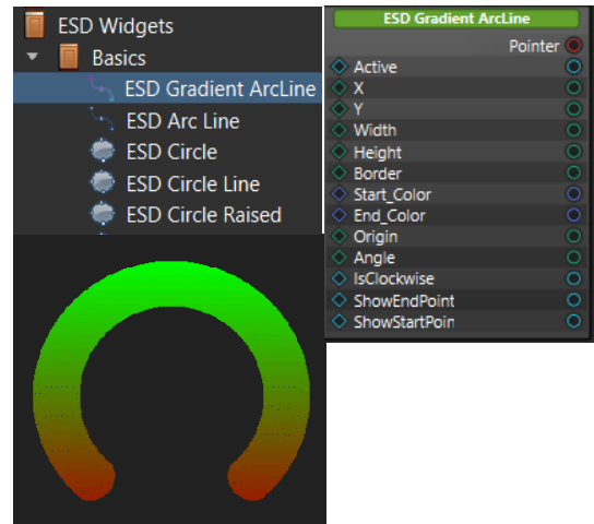
Figure 6 - ESD Gradient Arc Line Widgets
