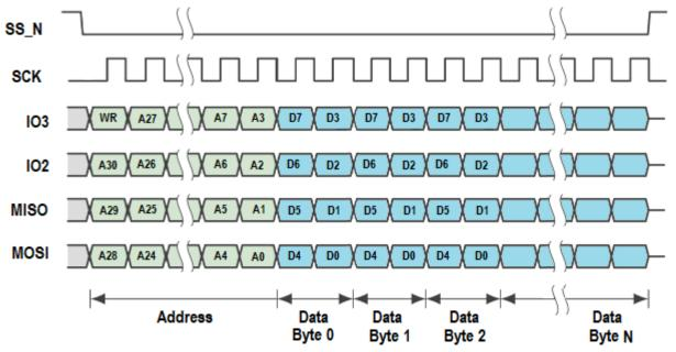
Figure 14 - Write Transaction Using Quad Channel Mode
