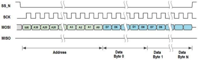
Figure 10 - Write Transaction Using Single Channel Mode
