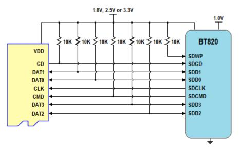
Figure 20 - Typical connection for SD Host Controller
