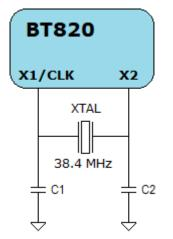
Figure 25 - Crystal Oscillator Connection
