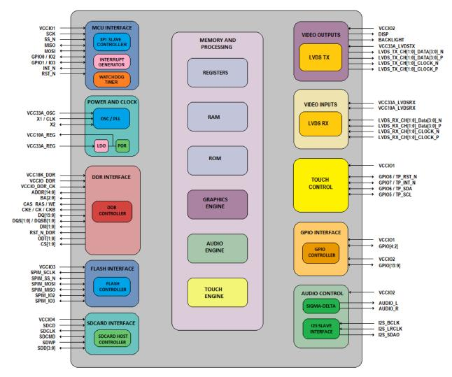
Figure 1 - BT820 Block Diagram
