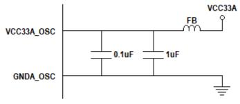
Figure 40 - Typical VCC33A\_OSC Application Circuit
