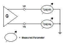
Figure 31 – Short-Circuit Measurement to Ground
