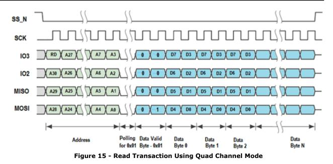
A transaction is considered to have started when SS\_N is driven to logic low and is considered to have ended when SS\_N is released to logic high. SS\_N high periods between transactions should have a minimum of 2 SCK cycles to ensure proper detection.
