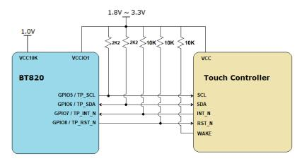
Figure 21 - Typical Touch Screen connection
