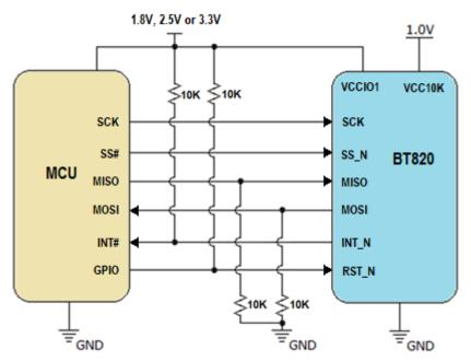
Figure 7 - QSPI Host Interface Using Single SPI Connection
