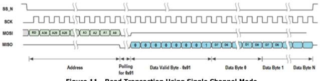
Figure 11 - Read Transaction Using Single Channel Mode
