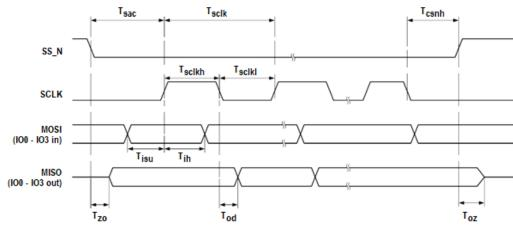
Figure 35 - Quad Host interface I/O Timing Diagram
