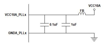
Figure 41 - Typical VCC10A\_PLL Application Circuit
