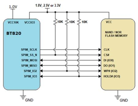
Figure 19 - Typical Connection for Flash Memory
