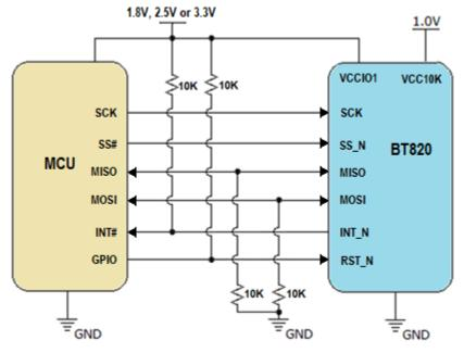
Figure 8 - QSPI Host Interface Using Dual SPI Connection
