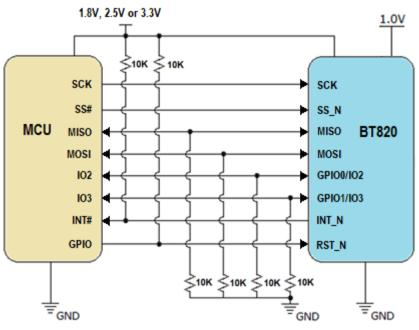
Figure 9 - QSPI Host Interface Using Quad SPI Connection
