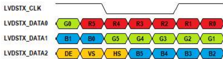
Figure 6 – JEIDA / Format 1 Mapping for 18-bit RGB
