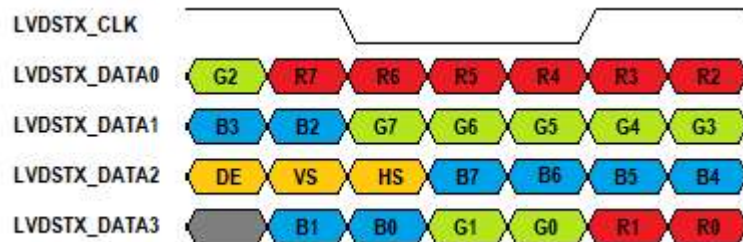
Figure 5 – JEIDA / Format 1 Mapping for 24-bit RGB
