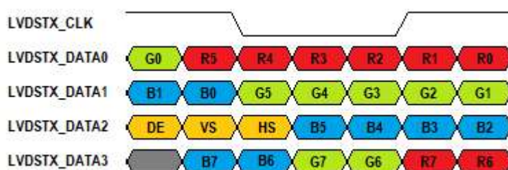
Figure 4 – VESA / Format 2 Mapping for 24-bit RGB
