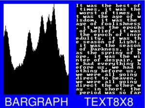
**BARGRAPH** – render data as a bar graph. Looks up the x coordinate in a byte array, then gives an opaque pixel if the byte value is less than y, otherwise a transparent pixel. The result is a bar graph of the bitmap data. A maximum of screen widthx256 size bitmap can be drawn using the BARGRAPH format. Orientation, width and height of the graph can be altered using the bitmap transform matrix.
