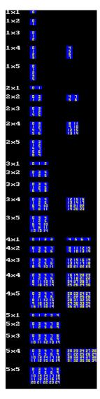
ASTC bitmaps in flash must be 64-byte aligned. This means that multi-celled bitmaps must have a size which is a multiple of 4 blocks. In particular fonts in flash must use a multiple of four blocks per character. Note that only bitmaps with multiple-of-four size have cell 1 shown.
