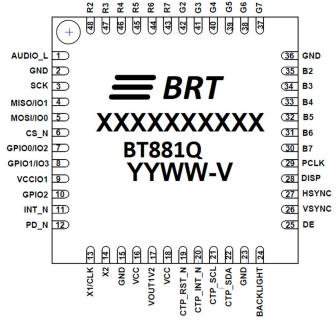
Figure 3-2 Pin Configuration BT881 VQFN-48 (top view)
