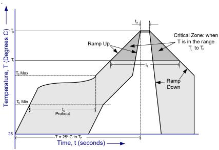
Figure 8-3 BT880/1 Solder Reflow Profile
