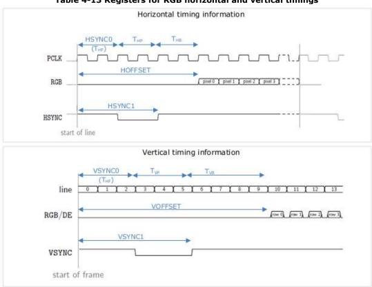
Figure 4-7 RGB timing waveforms
