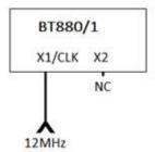
Figure 4-6 External clock input
