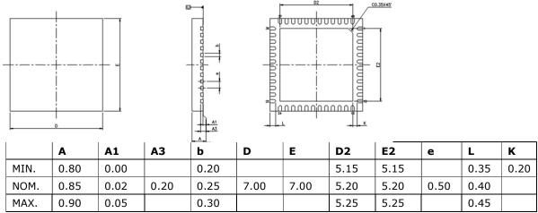
Figure 8-2 VQFN-48 Package Dimensions
