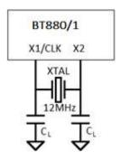
Figure 4-5 Crystal oscillator connection
