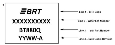
Figure 8-1 Part Marking Example
