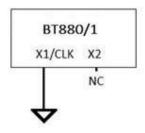
Figure 4-4 Internal relaxation oscillator connection
