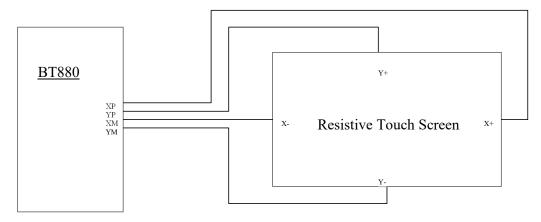
Figure 4-8 Resistive Touch screen connection
