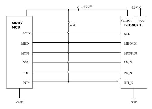
Figure 4-2 Single/Dual SPI Interface connection
