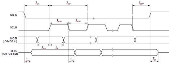
Figure 6-1 SPI Interface Timing
