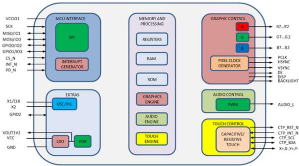
Figure 2-1 BT880/1 Block Diagram
