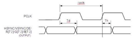
Figure 6-2 RGB Interface Timing
