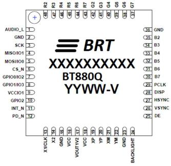
Figure 3-1 Pin Configuration BT880 VQFN-48 (top view)
