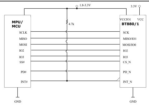
Figure 4-3 Quad SPI Interface connection
