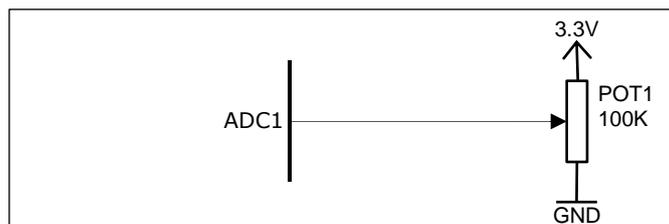
**Figure 9 - Circuit Diagram for ADC Examples**
