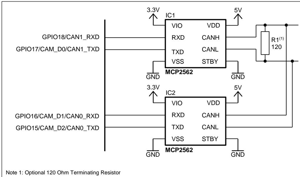
**Figure 10 - Circuit diagram for CAN Examples**
