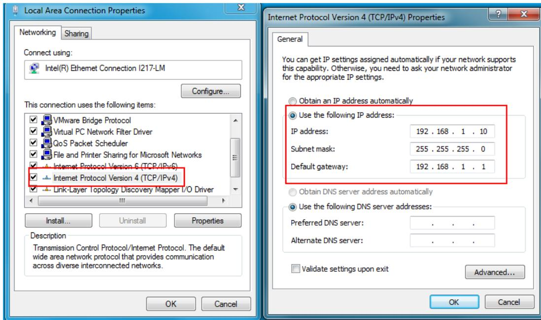
**Figure 18 - Host PC static IP configuration**
