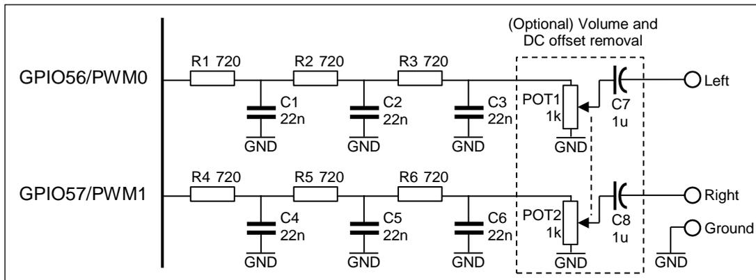
**Figure 26 - PWM Low Pass Filter**
