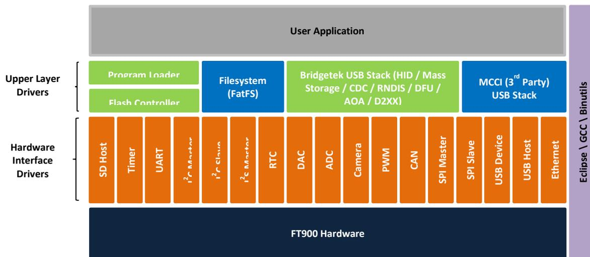
**Figure 1 - FT90X Series Interface Driver Support**
