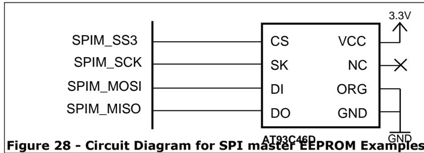
**Figure 28 - Circuit Diagram for SPI master EEPROM Examples**
