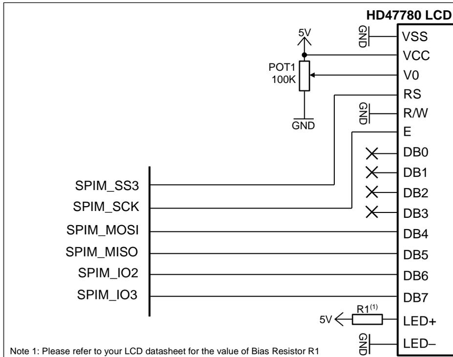
**Figure 29 - Circuit Diagram for SPI Master Example 3**
