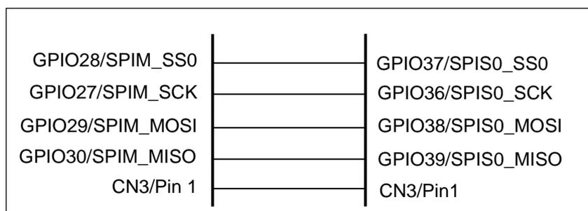
**Figure 30 - Circuit Diagram for SPI Slave Examples**
