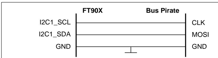
**Figure 25 - Circuit Diagram for I2C Slave Examples**
