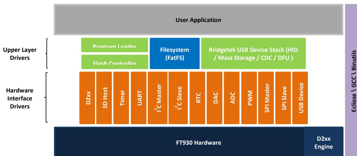
**Figure 2 - FT93X Series Interface driver support**
