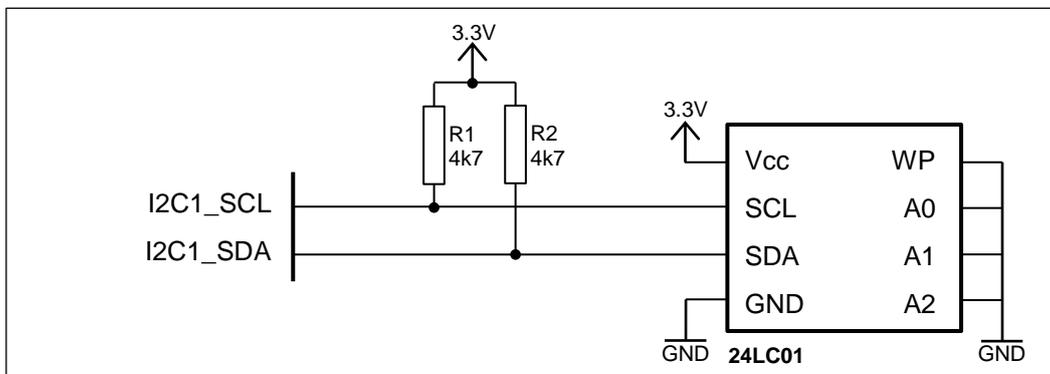
**Figure 24 - Circuit Diagram for I2C Master Examples**
