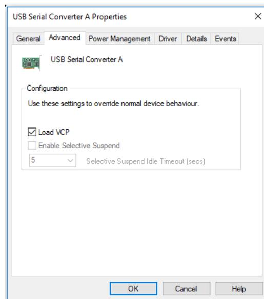
**Figure 8 - USB Serial Converter Properties**
