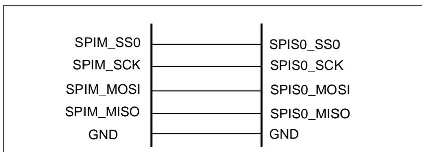
**Figure 27 - Circuit Diagram for SPI Master Examples**
